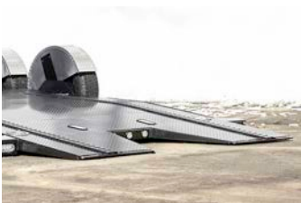
Split Tail Knife Edge Rear With 8.8° Loading Angle For The First 5', Then 4°
