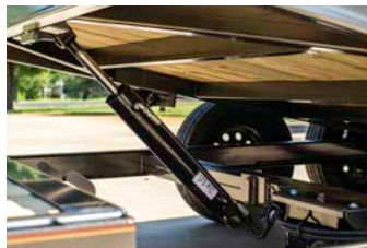
3X16 Cushion Cylinder with Lock-Out Valve
